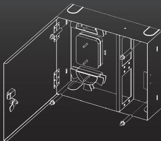
Step 1. Mount the enclosure on the wall.
